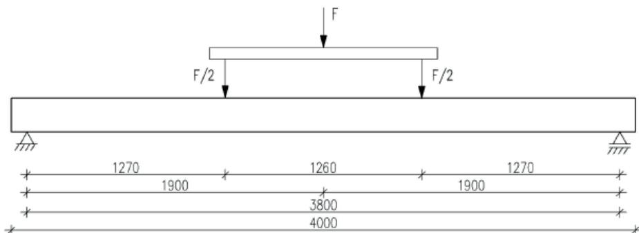
Fig. 10. Scheme of the test stand [15].
