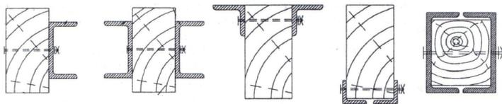
Fig. 6. Strengthening of wooden beams using steel profiles [4]
