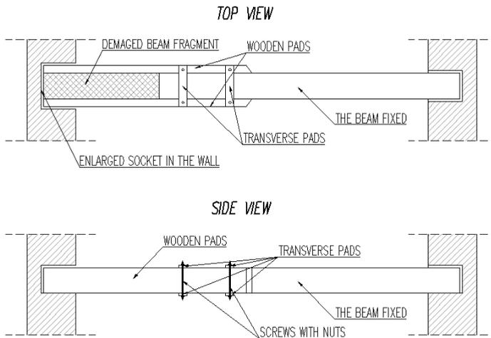
Fig. 5. Strengthening of wooden beams using wooden pads [4]
