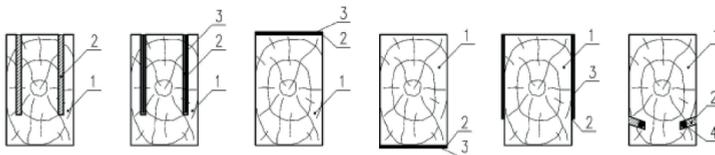
Fig. 7. Strengthening of wooden beams using steel sheets and steel rods [5]; 1-wooden beam reinforced, 2- epoxy composition, 3- metal sheet, 4 –steel rod
