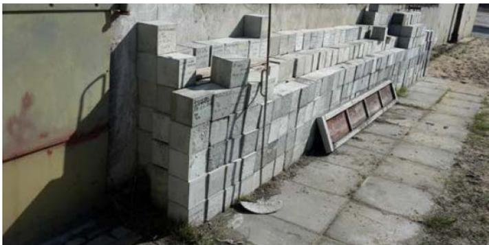
Fig. 2. Incorrect storage of concrete samples. *Source:* [8]
