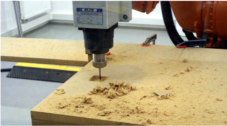
Fig. 4. 6-axis KUKA KR 60 HA robot arm during the milling process. Source: [Marcin Giedrowicz]
