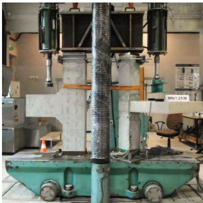
Fig. 3. The test setup and location of strain gauges. Source: own study
