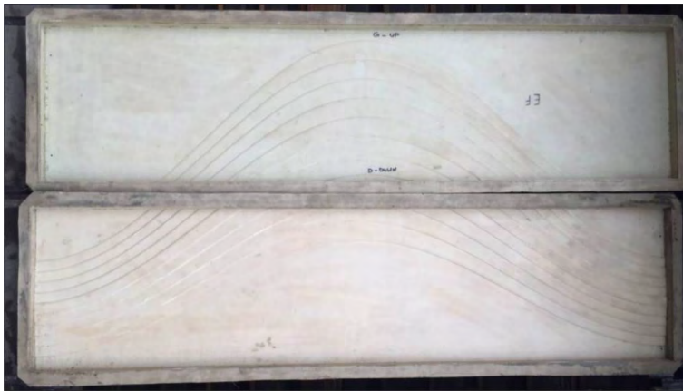
Fig. 10. Fibreglass mould [9] of “Wave” – a negative form before concrete filling process. Source: [Marcin Giedrowicz]
