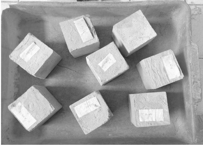
Fig. 7. Mortar cube specimens. *Source:* own study
