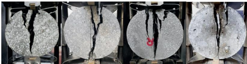
Fig. 8. Examples of the specimens' failure after the tensile splitting test, concrete with crushed granite aggregate (from the left): cylinder  $150 \times 300$ ,  $C/W = 1.8$ ; cylinder  $150 \times 150$ ,  $C/W = 1.8$ ; cylinder  $150 \times 300$ ,  $C/W = 2.6$  and cylinder  $150 \times 150$ ,  $C/W = 2.6$
