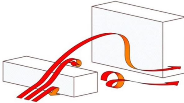
Fig. 5. The downwash vortex effect. Adapted from [4]
