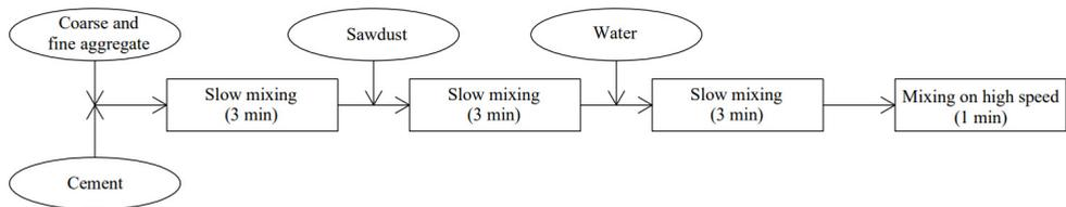
Fig. 5. Diagram of sawdust concrete mix formation. *Source:* [1]
