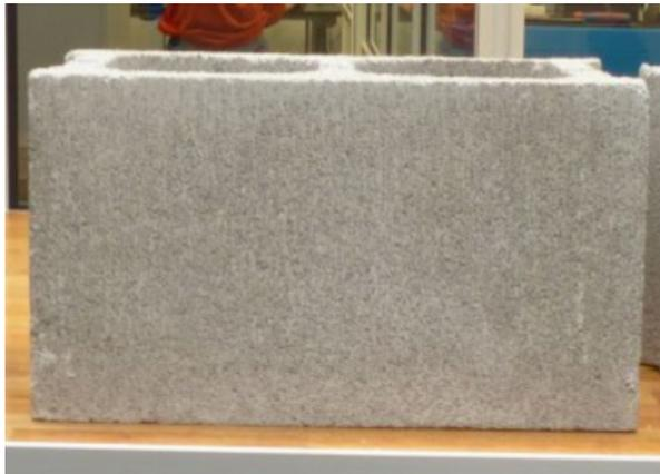
Fig. 3. Sawdust concrete block with 5% fine sawdust. *Source:* [16]
