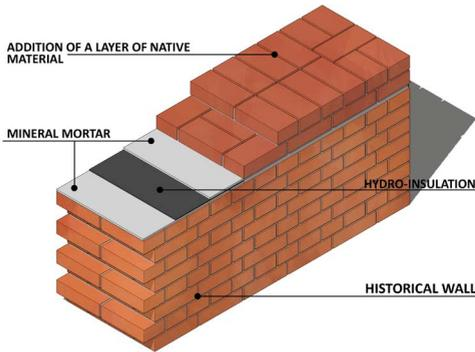
The insertion of an insulation layer in the form of roofing felt or metal sheeting is a cheap and quite effective way of protecting the wall topping. It is also a much better solution than to merely over-brick the wall topping. Insulation gives additional protection to the old masonry, provides a separating layer and makes the solution reversible. In contrast, brickwork provides a pressure layer for the insulation and is considered a lost layer that needs to be restored periodically.
