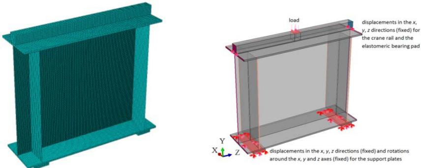
Fig. 5. The mesh and the boundary conditions used in the numerical model
