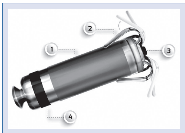
Figure 1. Build of the Micra AV; 1 — capsule; 2 — fixation tines; 3 — stimulation cathode; 4 — stimulation anode.
