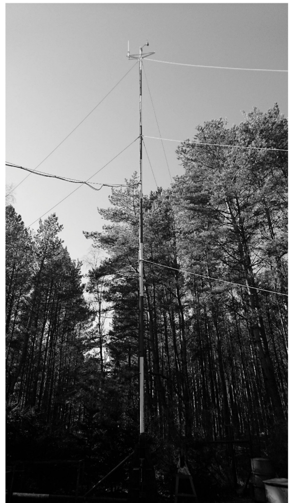
Figure 3 Anemometer on top of a mast at CRS Lubiatowo.
