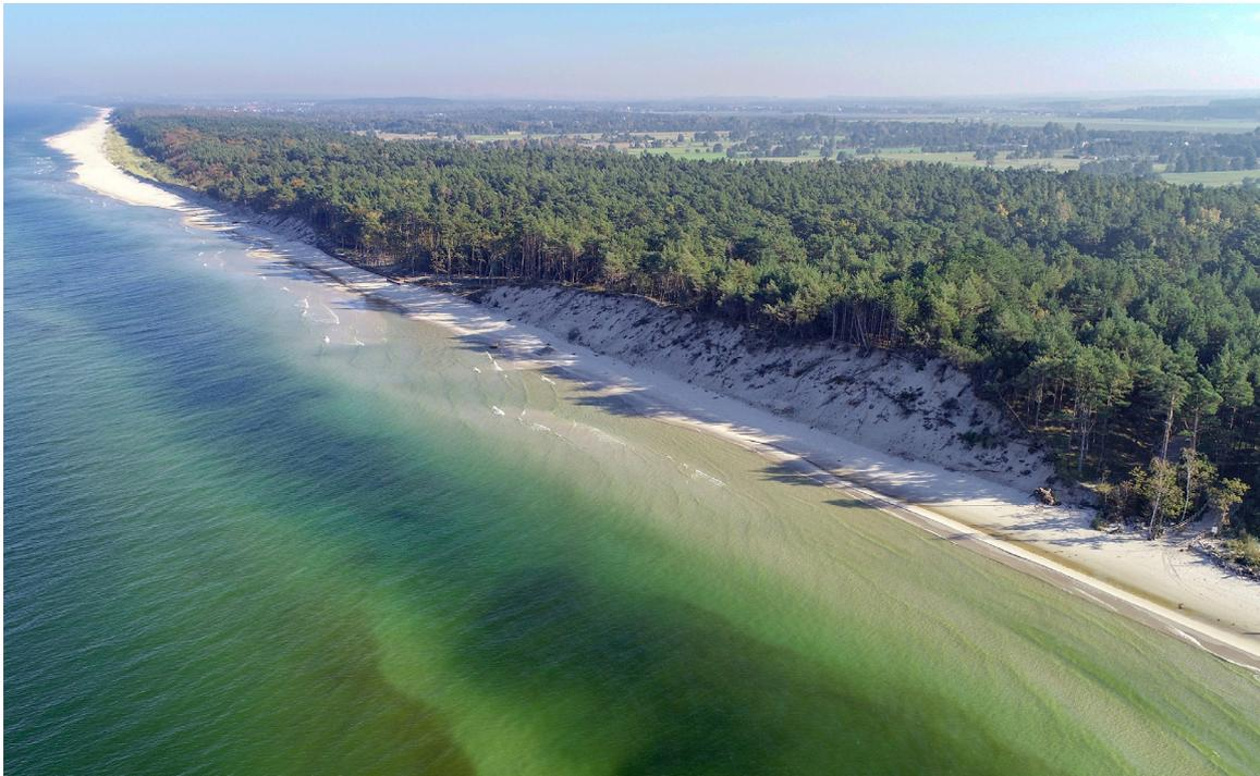
**Figure 6** Aerial view (towards the ESE) of the study area (photo by: M. Olkowicz, 2018). No foredune within the “hot spot”; visible: very narrow beach in front of the erosional undercut in the remains of the parabolic dune.
