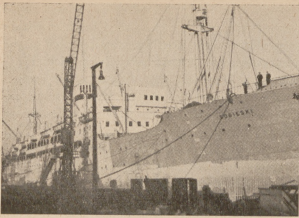
11,000 BRT Motor Liner „Sobieski“ Refitted from Troopcarrier to Passenger & Cargo Liner in the Northern Shipyard in Gdańsk.
